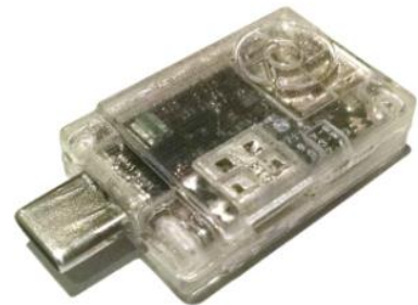
This page describes a USB-PD sniffing dongle with Type-C connectors.
