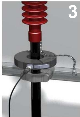
HFCT around cable ( i- + i+ = 0 )
