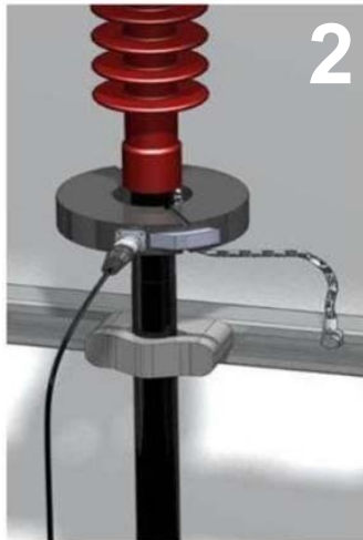
HFCT on cable with Earth brought back through ( i+ )
