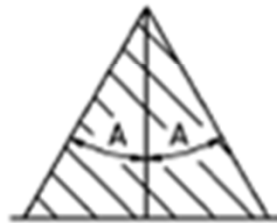
SINGLE MAST OR SHIELD WIRE
