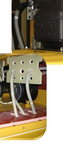
Voltage clamping module for CTs mounted in main or neutral box on hazardous applications
