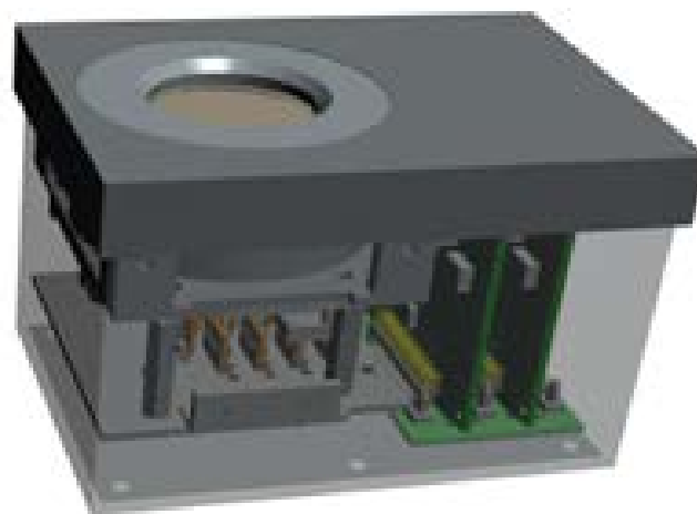
MErIT measures energy spectrum and intensity of electrons, protons, and H-Fe ions
