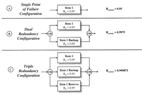
Figure 50.8 Improving System Reliability via Redundancy
