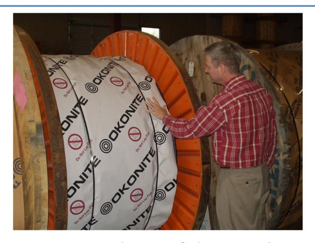
•The wrapper can indicate if damage has occurred.
