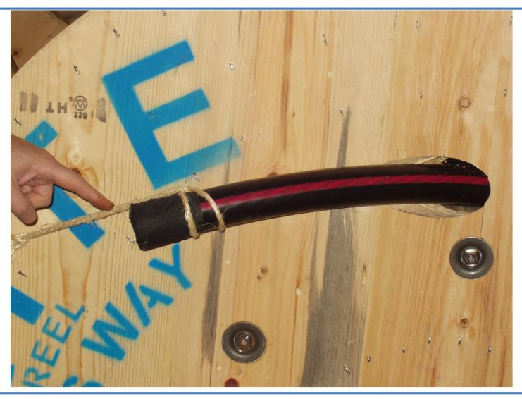
Do not pick up a reel by the flange (unless cable is removed). This can damage the cable and/or the flange.
