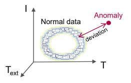
Can detect faults on any variable in the group
