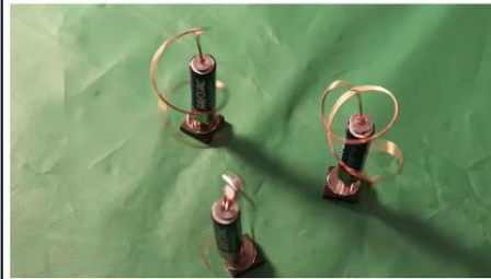
World' Simplest & DIY Motor (Homopolar Motor) for Outreach
